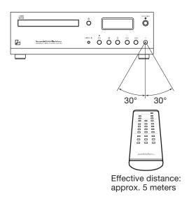
Do not expose the remote control infrared receiver to direct sunlight or strong light sources. That may cause malfunction.
