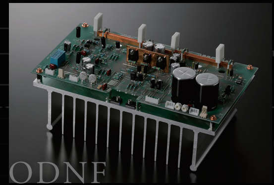
Power amplifier block of parallel module ODNF version 4.0
